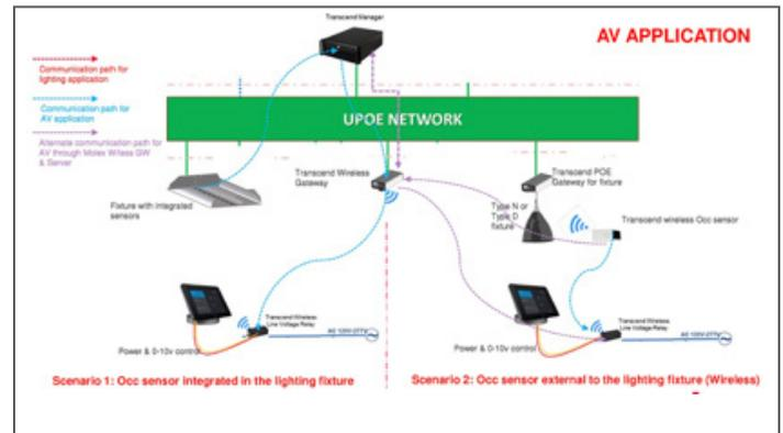
FIGURE 5: Diagram showing the connectivity and communication path for GP's AV application.
