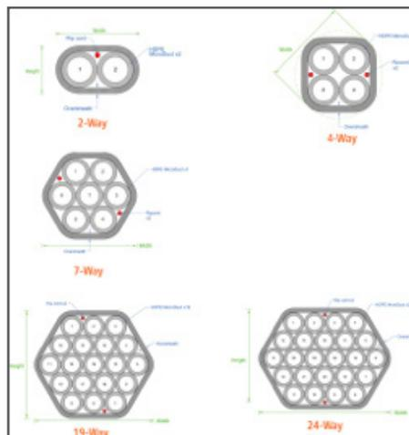
FIGURE 3: Microducts form permanent fiber pathways through which any type microcable (e.g., OS2, OM3, OM4, OM5, bend-insensitive) can be jetted or blown in a continuous splice-free (zero point of network failure) fiber run in and out of the network at typical speeds of up to 250 feet per minute using only two installers, thereby eliminating the high cost and time of large installation crews that would "pull fiber."<sup>2</sup>
