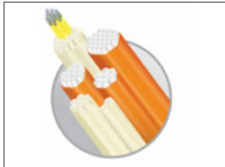
FIGURE 2: Providing flexibility in network infrastructure design, the microducts come in various bundled configurations containing 1 to 24 empty 8.5mm x 6mm inner microducts and include high density polyethylene (HDPE) OSP, riser, plenum, and low-smoke zero halogen options as dictated by the location in the network.<sup>1</sup>
